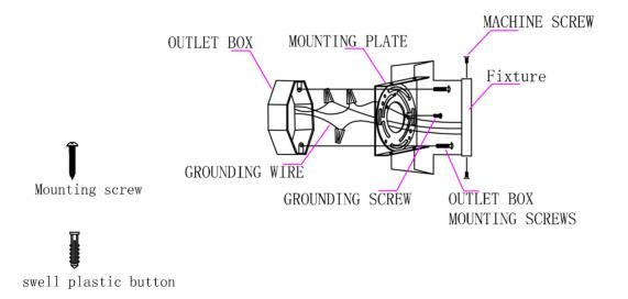
CAUTION :DISCONNECT POWER DURING INSTALLATION 1.) If you are replacing an existing fixture, disconnect and remove the old fixture. Expose the supply wiring from the outlet box.
